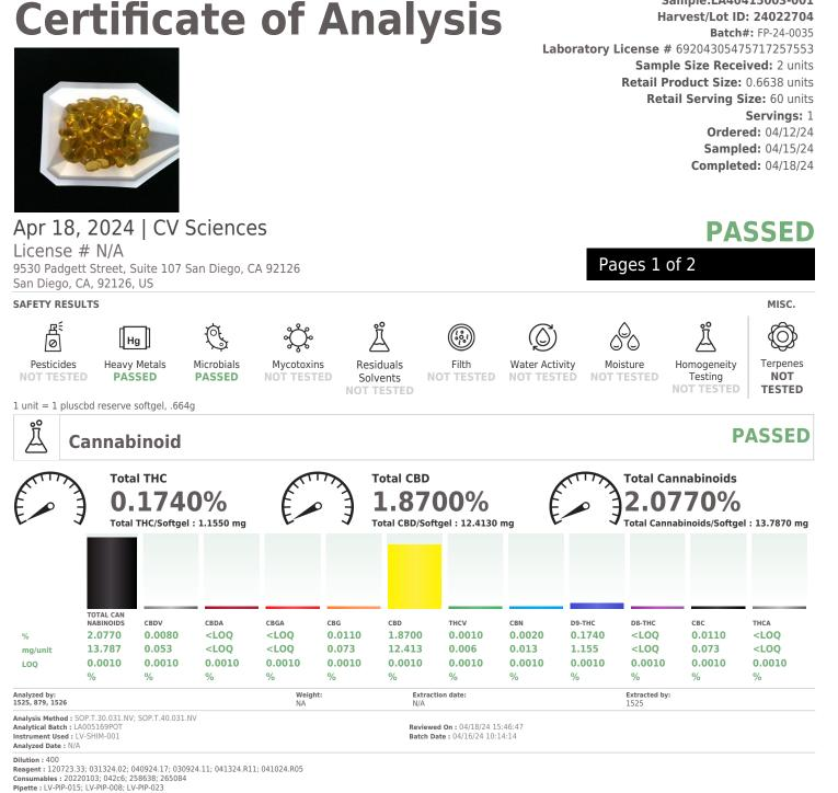
Cannabinoid analysis utilizing Ultra High Performance Liquid Chromatography with UV Detection (UHPLC-UV). Method SOP.T.30.031.NV for sample preparation and SOP.T.40.031.NV for analysis. Total THC = d8-THC + d9-THC + 0.877 \* THCA, Total CBD = CBD + 0.877 \* CBDA
